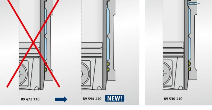
The engine manufacturer has modified the cylinder liner design.
